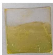
Fig. 2. BiVO<sub>4</sub> film synthesised *via* modified metal-organic deposition and spin-coated on to FTO-substrate glass.
